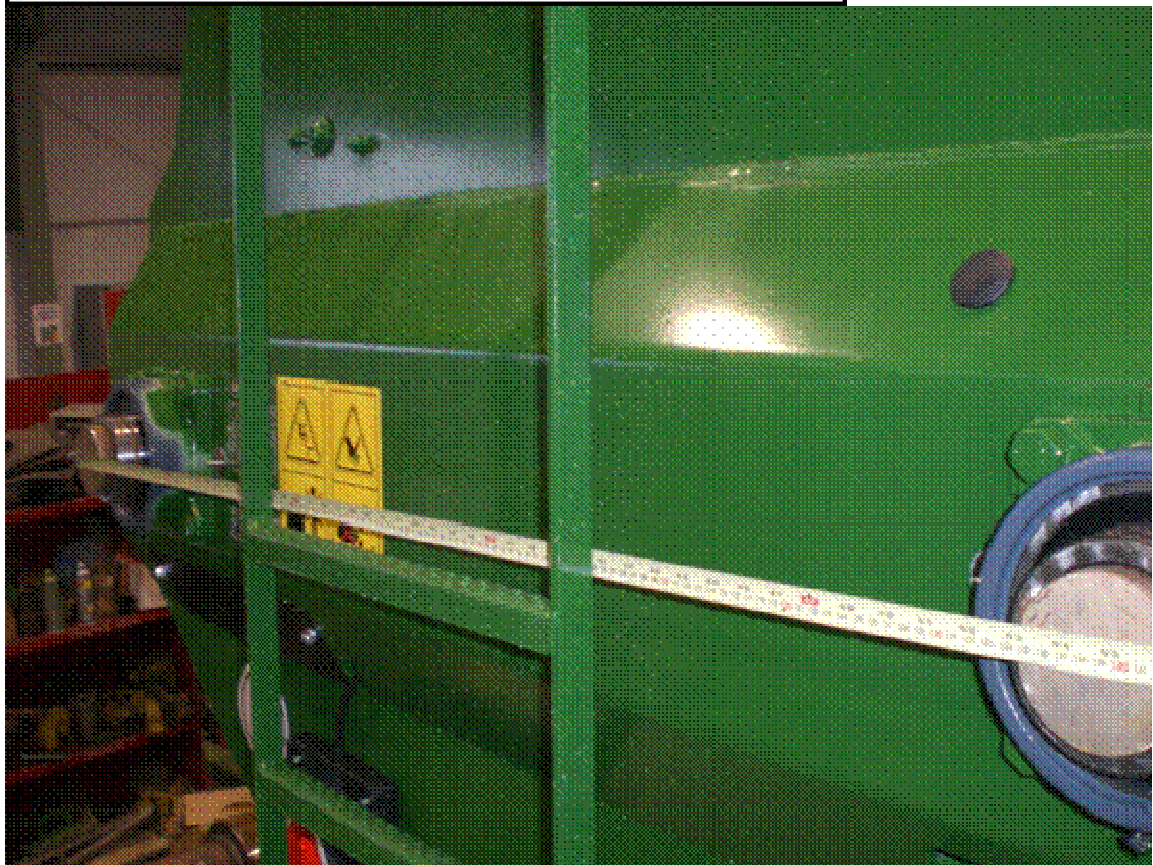
Photo 1 showing measurement technique to find shaft centres
