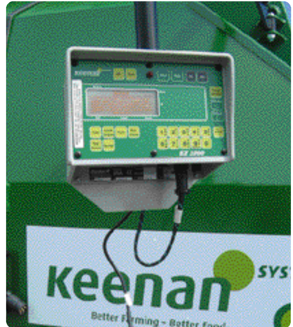
Photo 3 - Display cable disconnected from weighbox
