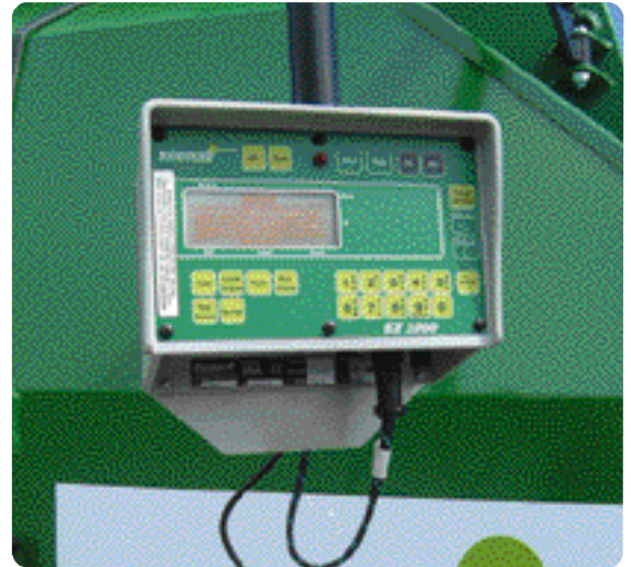
Photo 8 - Disconnected display cable
