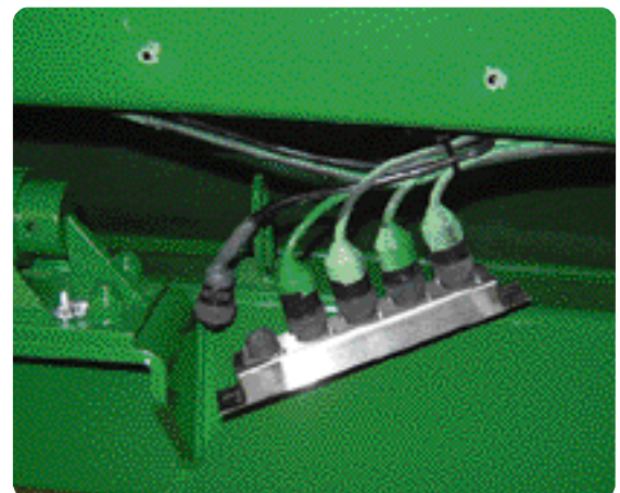
Photo 4 - Display cable disconnected at junction box
