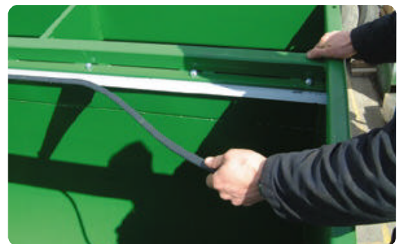
Photo 2 - Beaded strip fitted for protection from top knife
